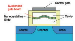
A schematic diagram of a nanoelectromechanical nonvolatile memory device that incorporates nanocrystalline-Si dots
