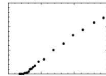
Light output characteristic of membrane DFB laser under RT-CW conditions
