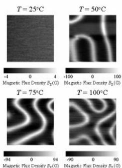
Scanning Hall probe microscopic images of a  $50 \mu\text{m} \times 50 \mu\text{m}$  area of a garnet film under an external perpendicular magnetic field of 150 Oe and at varied temperature
