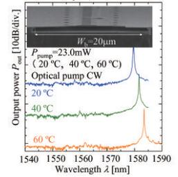
The lasing spectra of an air-bridge membrane DFB laser.
