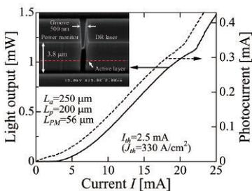
The  $I$ - $L$  and photocurrent characteristics of the integrated device.
