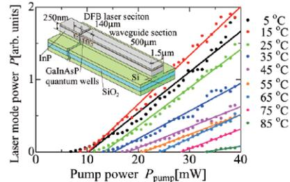
The lasing characteristics of a membrane DFB laser integrated with a silicon-on-insulator waveguide.
