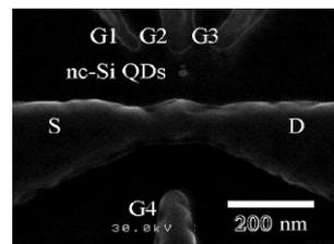
A scanning electron micrograph of a SET into which nanocrystalline quantum dots have been integrated.
