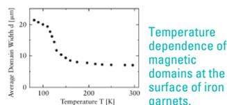
Temperature dependence of magnetic domains at the surface of iron garnets.
