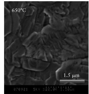
A surface scanning electronic microscopic image of CIGS film grown with cracked selenium.
