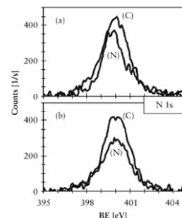
Hybridization results showing the high resolution spectra of the N 1s signal for complementary (C) and noncomplementary (N) samples: (a) surface, after immobilization of the thiolated probe molecules; (b) solution, before the surface immobilization.
