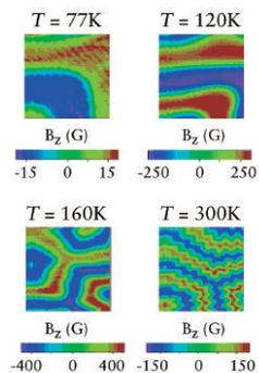
Visualization of magnetic domains at the surface of iron-garnet film.
