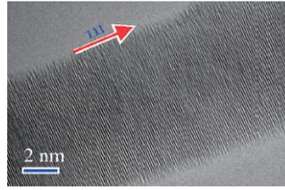
free and have single-crystal cores. Large-diameter silicon nanowires, on the other hand, are prone to a high density of defects.
