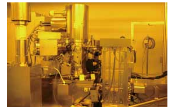
New electron beam lithography system at QNERC with a choice of 25, 50 or 100 kV acceleration voltages.
