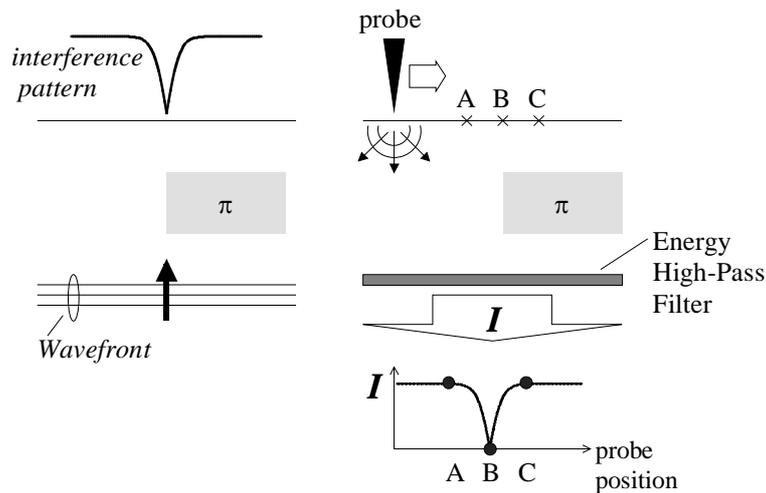
**Figure 1:** A conceptual figure to explain basic principle of our new SHEM
