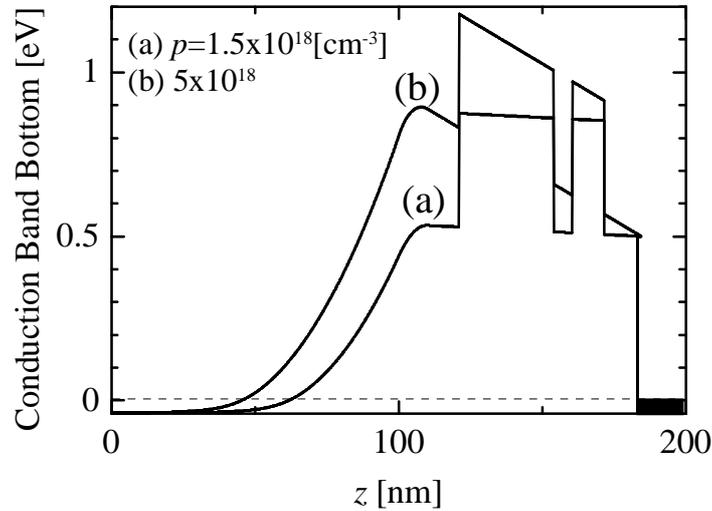
**Figure 2:** Calculated band profile inside the device
