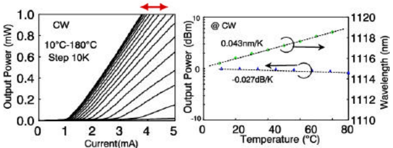
Fig. 5 Lasing characteristics of GaInAs/GaAs VCSEL grown on (311)B substrate
