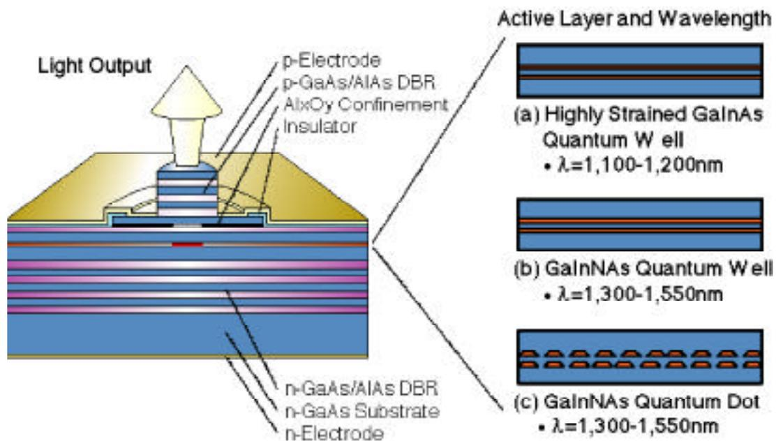
Fig. 4 Long wavelength VCSEL possibility on GaAs substrate
